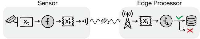
Figure 2. Workflow of the sensor-edge system implementing the consistent detection workload division strategy. Here x_t and x'_t = f_1(x_t) denote an input observation and its partially processed reduced version, respectively; f_1 and f_2 stand for the on-sensor and on-edge portions of the detector algorithm f(x_t) = f_2(f_1(x_t)) implemented by the system. Green checkmark represents arrival at the decision to accept an observation as a detection, while red cross signifies the rejection.
